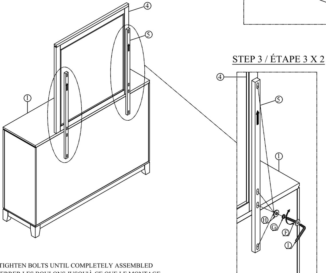
\*\*DO NOT TIGHTEN BOLTS UNTIL COMPLETELY ASSEMBLED
