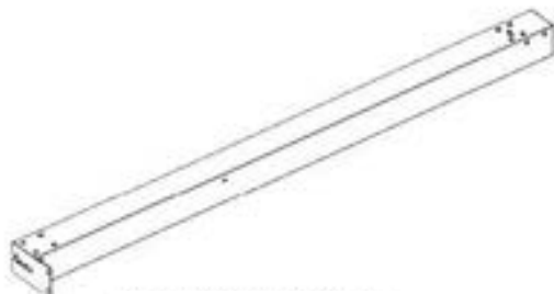
P03 POTEAU - A4M04969 (x1) 87 7/8 po x 7 7/8 po x 4 3/4 po (120 x 200 x 2232)
