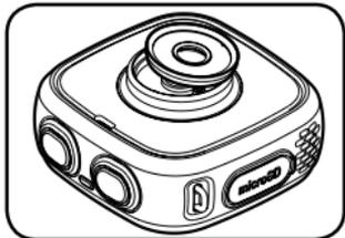
3. After removing this plate, you will find two screws. Use a screwdriver to remove them.
