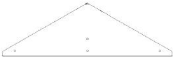
K01 MOLDURA DE TOPE - W4L20896 (x1) 5/8" x 51/4" x 16-9/16" (16 x 134 x 420)
