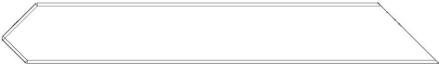
F18 SOPORTE ANGULAR - W4L21307 (x1) 1-7/16" x 2-3/8" x 17" (36 x 60 x 432)
