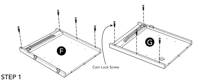
Insert Cam Lock Screws into pre-drilled holes of Side Panels (F) and (G). (See Figure 1)
