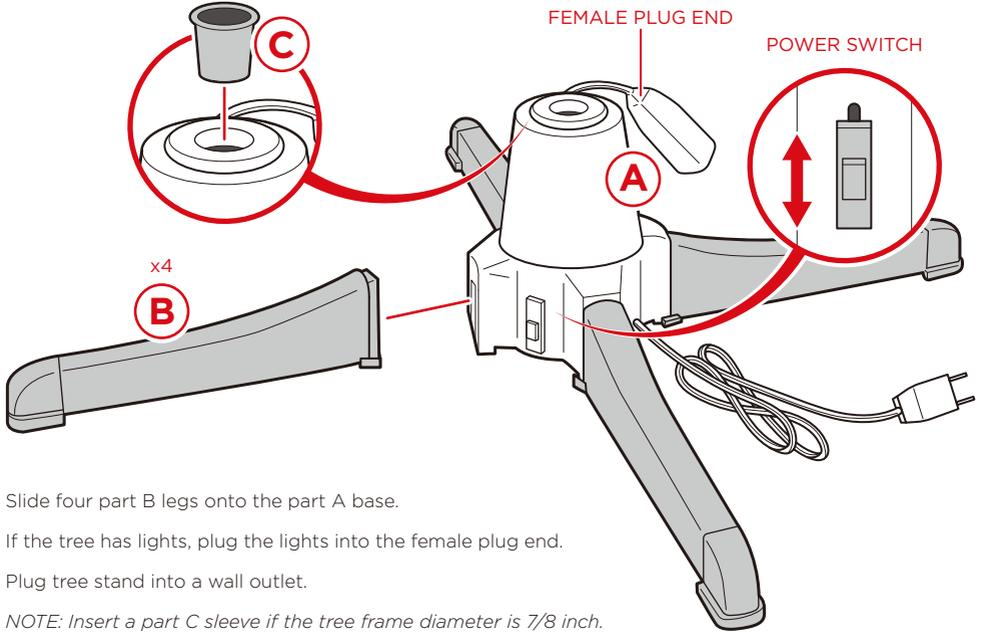
Slide four part B legs onto the part A base.
