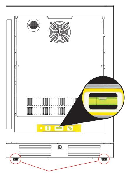
Rotate to raise or lower the LEVELING LEGS located at each of the four corners until all four legs are seated firmly on the floor and the interior floor of the unit is level both front to back and side to side.
