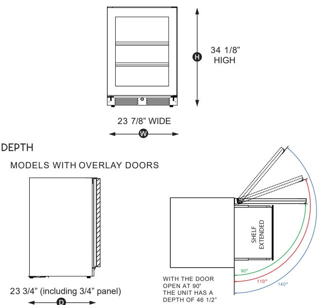
CUSTOM OVERLAY PANELS MAY ADD UP TO 3/4" IN OVERALL DEPTH YOUR CHOICE OF CABINET HANDLES WILL ALSO ADD DEPTH AND REQUIRE CLEARANCE SPACE IF INSTALLED NEXT TO A WALL TO OPEN.
