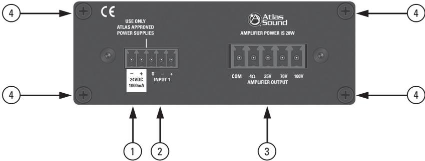
TSD Input/Output connections are removable for easy system wiring. The connectors have a 3.5mm pitch between pins.
