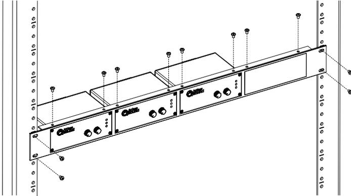
2. TSD-RMKHR Half Width Rack Mount Kit - AtlasIED offers an optional rack mount kit that can be used in half width rack applications including the AtlasIED WMA-HR and AWR-HR models. The TSD-RMKHR can support up to two TSDs. Included is an extra blank panel to fill one of the spaces if only one TSD is being used.
