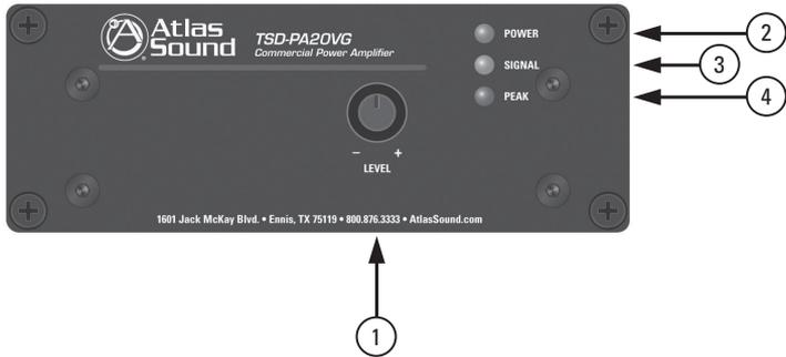
1. **Input Level Control** - Determines the output level at the loudspeakers on the PA20VG. Turn clockwise to increase the signal level and counter-clockwise to decrease the level. **Note:** The Input Level Control knob can be removed and replaced with a supplied security cover to prevent unauthorized adjustment.
