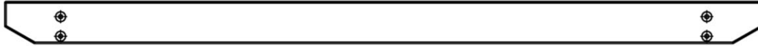
E01 PLANCHE DE GARNITURE - W4L22345 (x2) 1 7/16 po x 3 3/8 po x 60 3/8 po (36 x 86 x 1534)
