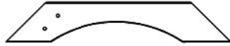
D12 | CALE ANGULAIRE COURTE - W4L13483 (x2) 1 3/8 po x 5 1/4 po x 29 3/4 po (36 x 134 x 755)
