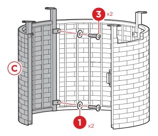
Flip the assembly and attach the part F tank holder with four part 3 screws and four part 1 washers. Return the assembly to the upright position before proceeding to the next step.
