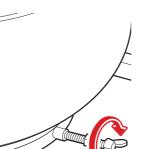
Turn the release valve on the tank counterclockwise to release the gas, then close the door and enjoy.
