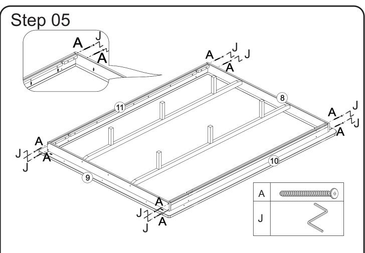
Secure parts (10,11) to parts (8,9) with screw (A) and hex key (J)
