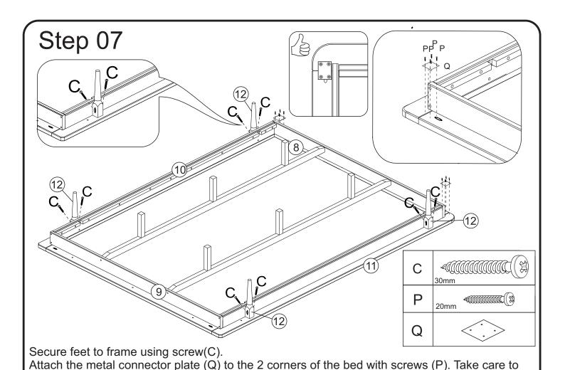
aligne the plate over the sean of the two parts, as shown in the drawing, before seguring in place
