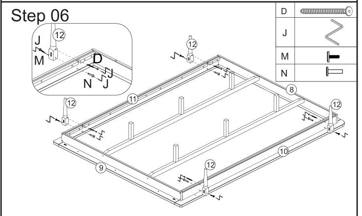
Attach Feet (12) to frame parts (10,11) using screw (M) and Union Screw (N). Union Screw (N) Should be on the inside of the bed frame, with screw (M),on the outside of the leg. Tighten by using with hex key(J) on both ends of the screw at the same time. The use Screw (D) and hex key (J) to secure legs(12).
