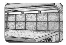
3 To terminate last APS- TR Series, use wire nuts on ends of wires. Snap cover in place, and turn power on. Firmly insert plug straight into receptacle, applying equal pressure to both blades at the same time. Gently rock plug, if needed.
