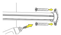
3. Slide end flanges onto the Lighted Closet Rod and place the rod on the shelf support center bracket. Slide the end flanges to the wall and mount using the providing screws, making sure the rod is level.
