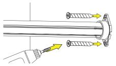
**5.** Using the provided screws, mount each end flange in desired location.
