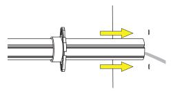
**4.** Slide end flanges to the wall, making sure the wire exists through the wire groove on the back of the end flange.
