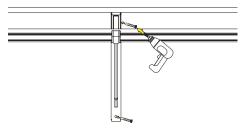
**1.** Center bracket under shelf and secure to the wall using the screws provided.
