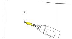
1. Locate desired height for Lighted Closet Rod. Mark and pre-drill holes for end flanges on both sides of closet.
