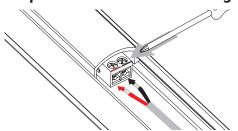
1. Strip wires and remove frosted lens from the fixture. Use #1 Philips to loosen the terminal screws on the EZ Connector. Connect wire into terminals. Red wire to (+, DC24V, or WW) side marked in red, Black wire to (-, GND, or CW) side of tape marked in black; tighten screws. Replace frosted lens onto fixture.
