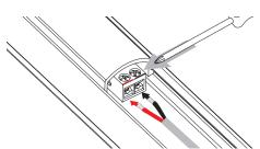
**2.** Follow instructions for wiring the Lighted Closet Rod to properly run lead wire through end flange.
