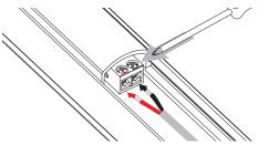
**2.** Connect wire to desired end, referring to step 2 in the Lighted Closet Rod instructions.
