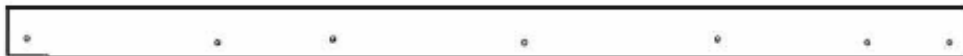
AD04 SUPPORT DE FAÎTE - W4L21553 (x1) 15/16 po x 4 po x 79 3/4 po (24x102x2025)
