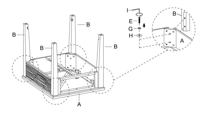
3 Attach the Shelf (C) to the Leg (B) by Connecting Metal (D) using Bolt (F), Spring Washer (G) and Flat Washer (H) with Allen Wrench (I). Fully tighten the bolts in this step.
