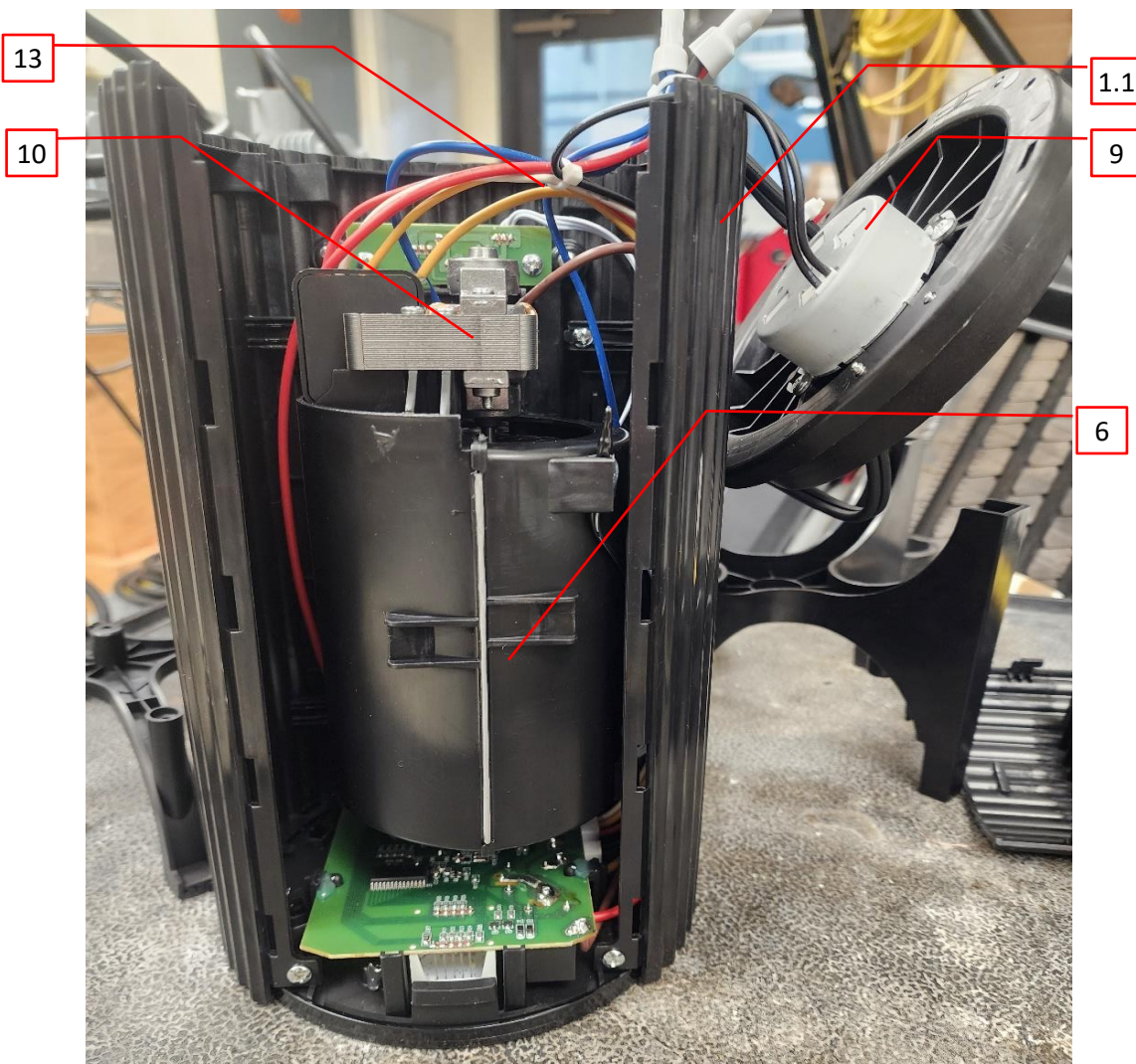
Photo 10 - Internal view of the of the CX16550 with most of the internal electronics installed
