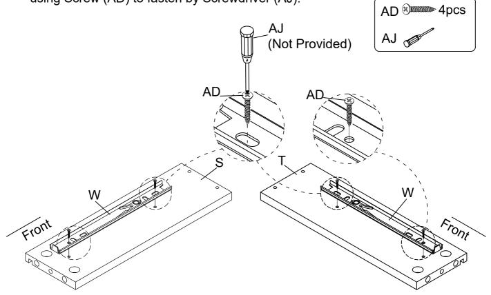
**15** Assemble Drawer Back Panel (U) to Drawer Left Panel (S) & Drawer Right Panel (T), using Screw (AC) to fasten by Screwdriver (AJ).
