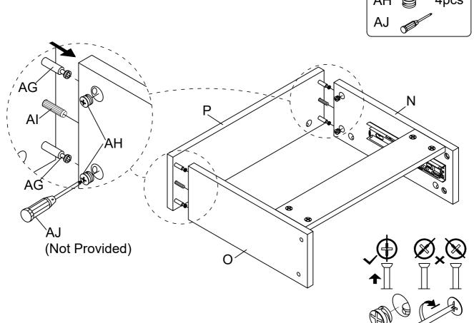
8 Assemble Bolt (AG) & Wood Dowel (AI) to Drawer Board - Top (M) by Screwdriver (AJ).
