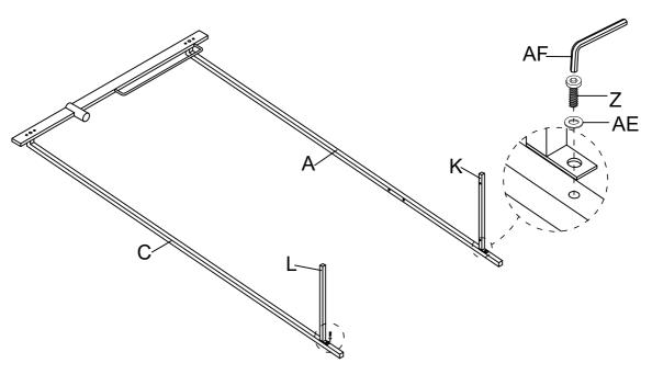
3 Assemble Post - Left Back (B) & Post - Right Back (D) to Cross Bar - Left / Right (K, L) and Top Panel (H), using Bolt (Z), Bolt (X) & Flat Washer (AE) to fasten by Allen Key (AF).
