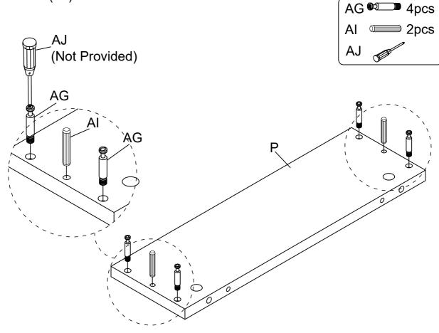
Assemble Drawer Board - Back (P) to Drawer Side Panel - LSF (O) & Drawer Side Panel - RSF (N), using Nut (AH) to lock with Bolt (AG), then fasten by Screwdriver (AJ).
