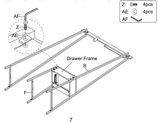
11 Assemble Bottom Support (I) & Cross Bar - Bottom (J) to Middle Frame (F) and Cross Bar - Left / Right (K, L), using Bolt (Z) & Bolt (X) to fasten by Allen Key (AF).
