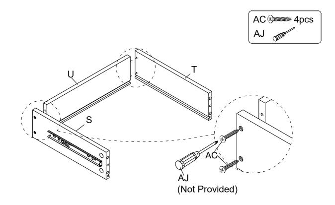
16 Assemble Drawer Board - Bottom (R) to Drawer Left Panel (S), Drawer Right Panel (T) & Drawer Back Panel (U).
