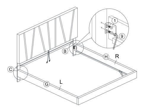
Do not fully tighten screws until assembly is complete and the bed is level.
