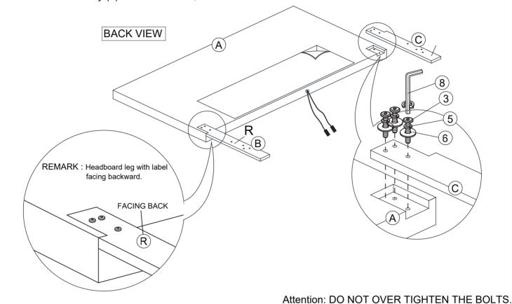
STEP 2: Assemble Headboard Support Rail (K) to the RSF Headboard leg (B) and RSF Headboard leg (C) by using Allen Key (8) with hardware 4, 5, and 6.
