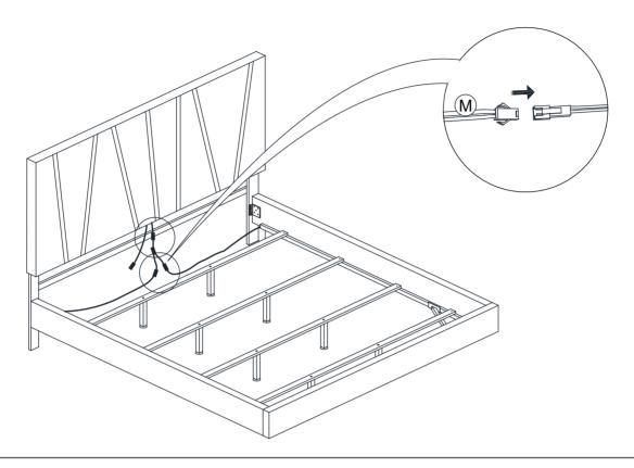
STEP 12: Connect the Plug (L) with the connecting wire on the Headboard (A).
