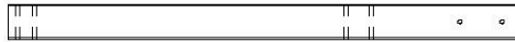
SP1 | SUPPORT DE POUTRE DE BALANÇOIRE - W4L15647 (x1) | 3 3/8 po x 3 3/8 po x 48 3/8 po (86x86x1229)
