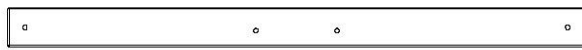
H14 | SUPPORT DE POUTRE DE BALANÇOIRE - W4L12719 (x1) | 1 po x 3 3/8 po x 50 1/4 po (24x86x1277)
