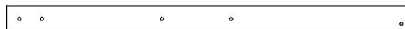
H10 PIED DU PORCHE - W4L14757 (x1) | 1 po x 3 3/8 po x 50 1/2 po (24x86x1282)
