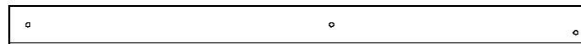
H11 PIED DU PORCHE - W4L14758 (x1) | 1 po x 3 3/8 po x 50 1/2 po (24x86x1282)
