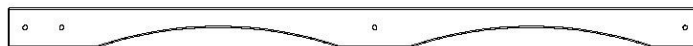
H28 | LISSE MURALE AVANT - W4L14774 (x1) | 1 po x 3 3/8 po x 60 1/2 po (24x86x1537)
