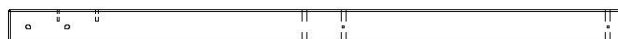
B7 | COIN FORT AVANT DROIT - W4L12686 (x1) | 3 po x 3 po x 53 7/8 po (76x76x1370)
