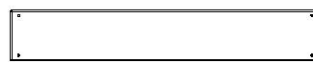
L1 | PLANCHE DE PLANCHER DU NID-DE-PIE - W4L14787 (x7) | 5/8 po x 4 3/8 po x 27 po (16x112x686)
