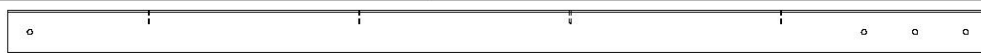
E74 (x2) RAIL DE BARRE DE SUSPENSION - W4L15732 1 3/8 po x 3 3/8 po x 77 1/8 po (36x86x1959)
