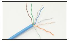
Separate each wire pair by untwisting.
