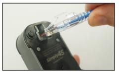
Insert the plug into the crimping socket on the Simply45 pass through crimper.
