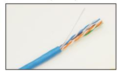
Be sure not to nick the wire insulation. If you nick the wire insulation, cut the cable off for all exposed wire cable pairs and re-strip the cable.
