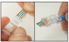
Hold the RJ45 plug upside down (strain relief clip facing down). Insert the wires into the back of the plug until they come out the front of the plug at least ½ inch (1.27cm).
