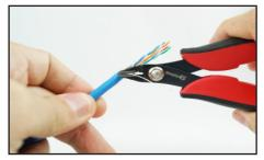
Trim off the "rip cord" at the cable jacket using Simply45 Flush Cutter (Part: S45-801).
