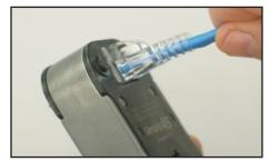
Make sure plug goes completely inside the crimping socket.
