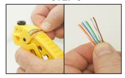
Straighten each wire conductor. Hint: Use wire straightening comb on top of Adjustable Stripper for faster straightening and less finger fatigue.
