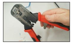
If the crimper handles do not release this means that you have not completed the crimping cycle. Simply squeeze the crimper handles further down until the crimper handles release.
