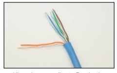
Align wires according to Termination Pattern either Type A or Type B. Hint: Hold wire so that the White Orange and Orange wires are closest to you and put in wire pattern order 1-8.
