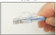
Then remove the terminated RJ45 plug from the crimping socket. Quickly inspect that all wires have been closely trimmed to the plug in the front.
