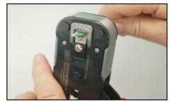
With one hand, firmly without stopping, compress the crimper handles all the way down in one steady non-stop motion.
