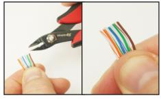
Using a flush cutter, trim the wires straight across so all of the wires are the same length.
