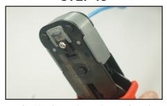
The Simply45 crimper is a ratcheted crimper. The crimper will not open up until the crimping process has been fully completed. This assures that the wire trims and pin sets have been done correctly.
