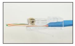
Push the plug as far down onto the cable until it stops inside the plug.
