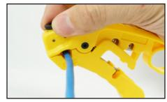
Using the Adjustable Cable Stripper (Part: S45-S01YL/S01BL), strip back the cable jacket about 1.5inches (3.8cm)
