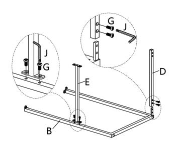
Insert Right Frame (C) to Rail (D) and Support Leg (E) using Bolt (G) with Allen Key (J). Note: At this stage, do not fully tighten the Bolts.
