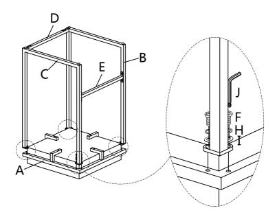
With assistance from an adult partner, stand the Stool up. Adjust the Pre-installed Levelers at the bottom of the Left Frame (B) and Right Frame (C) until the Stool levels with the ground.
