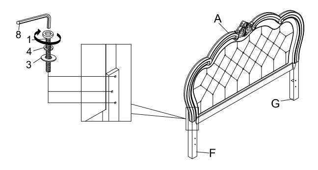
STEP 2 Assemble the HB cross bar (E) to HB legs (G & F) by using Allen Key (8) with hardware 1,3, and 4. \*TIGHTEN ALL THE BOLTS BY USING ALLEN KEY (8)
