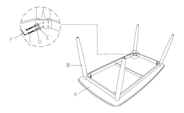
Stand table up on an even surface and check that it is balanced. If there is a slight wobble, apply downward pressure in the corner where a leg is uneven. Keeping pressure in that corner, tighten all bolts. If balanced, apply downward pressure evenly in the center and tighten all bolts. Do not over-tighten beyond hole depth.
