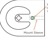
Leave set screw offset from hole in shade mount as shown
