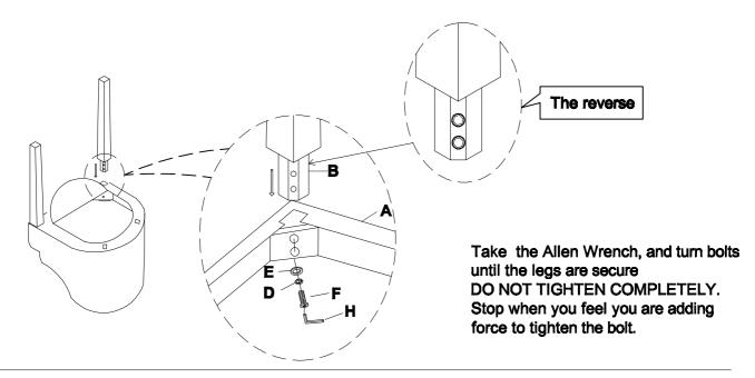
2 Attach the Back legs(C) to Seat(A) with Lock washer(D) and Flat washer(E) and Bolt(G) by Allen key(H).
