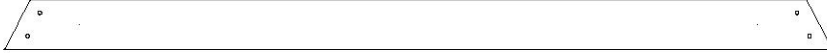
G50 | PLANCHE DE SOL - W4L16465 (x1) | 1 po x 5 1/4 po x 86 3/4 po (24 x 134 x 2 202)
