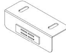
A2 MAGNET BRACKET - A4M03026 (x6) 1"x1 1/4"x3 1/8" (25x31x80)
