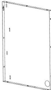
G5 BACK PANEL ASSEMBLY - A4M05477 (x1) 33 3/4"x25 13/16"x1 3/16" (30x655x857)
