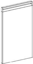
D5 DOOR ASSEMBLY - A4M05472 (x1) 22 3/8"x15 1/2"x7/8" (22x393.5x569)
