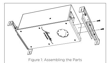
2. Tighten the screws just enough to allow movement for adjustment during installation.
