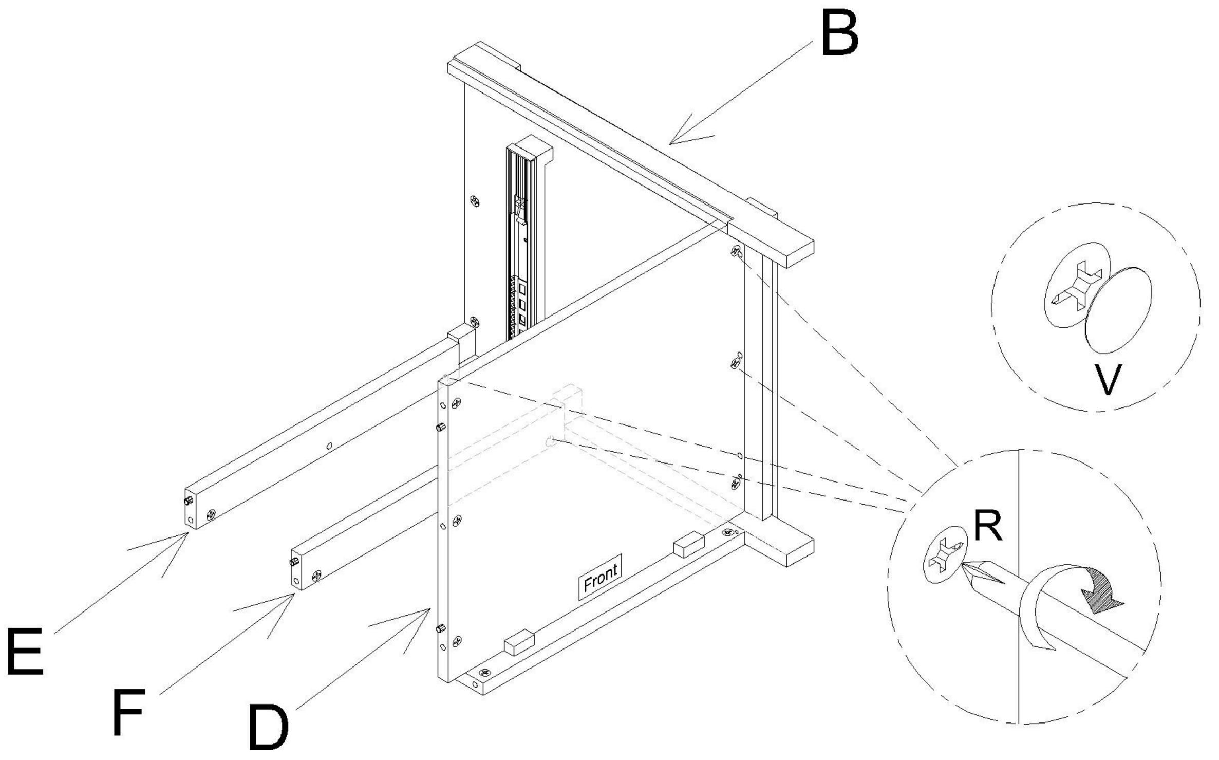
Attach Right Side Panel (C) to Top Bar (E), Center Bar (F) & Bottom Panel (D) and secure the Cam Lock (R) attached in the previous steps. Cover Cam Lock (R) with Cam Lock Cover (V).
