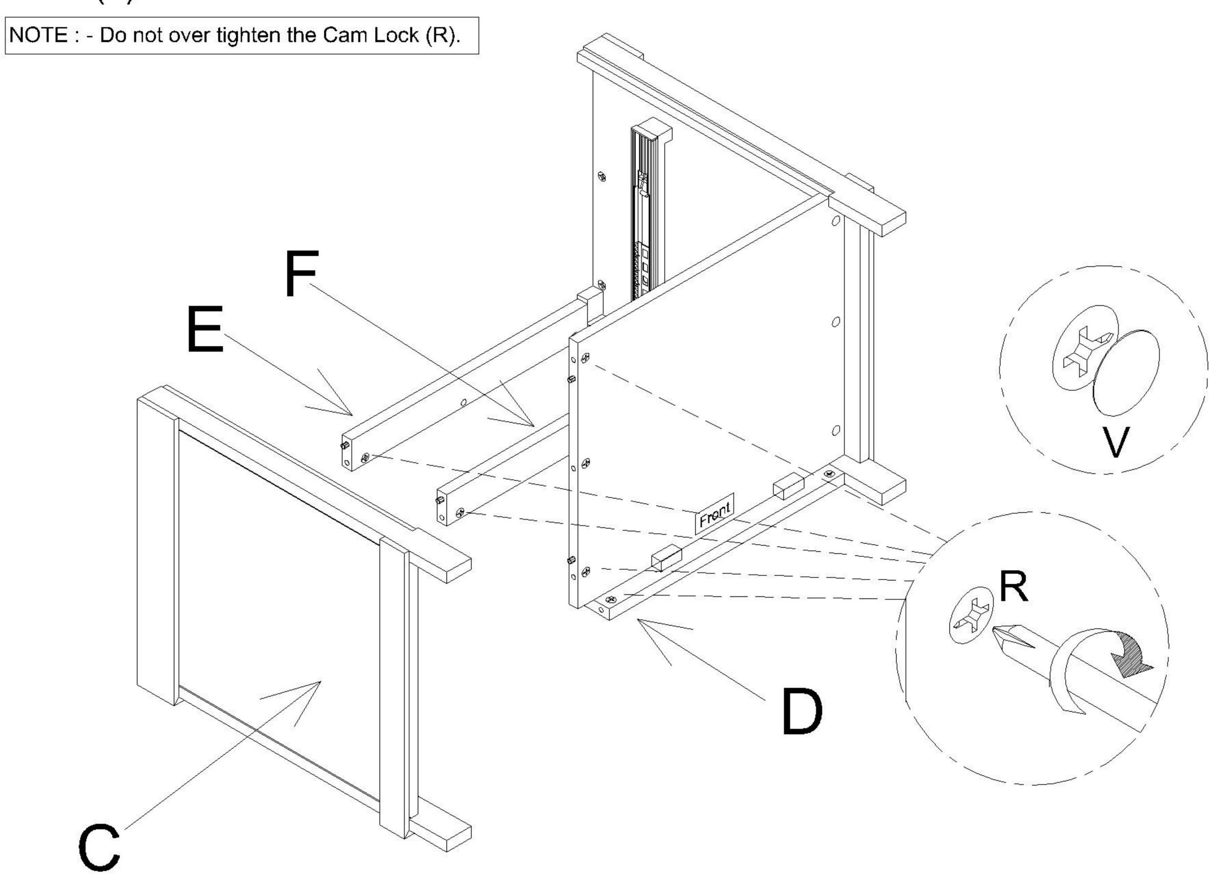
Attach Top Panel (A) to Left & Right Side Panel (B & C) and secure with the Cam Lock (R) attached in Step 2. Cover Cam Lock (R) with Cam Lock Cover (V).
