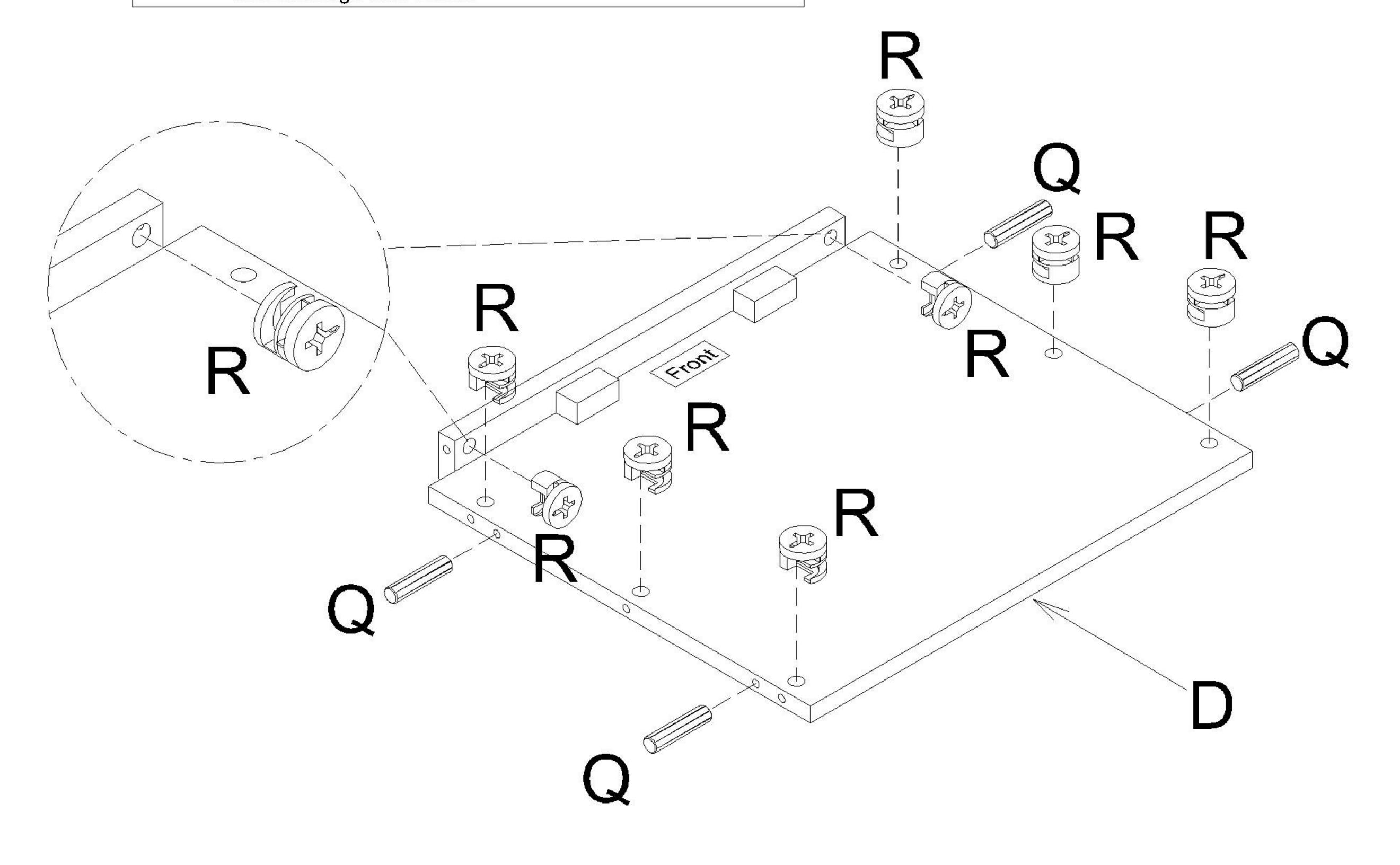
Attach Dowel (Q) and Cam Lock (R) to Top Bar (E) & Center Bar (F).
