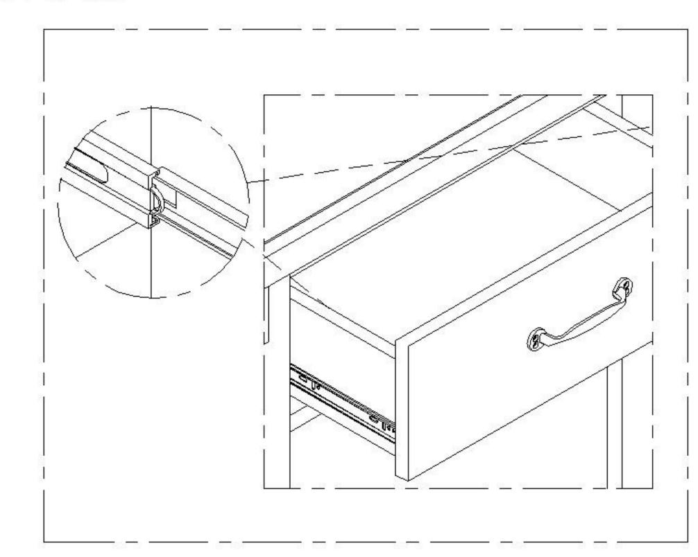
NOTE: Align and pull/push the triggers on both sides of drawer box into the metal track on interior side of side panel.
