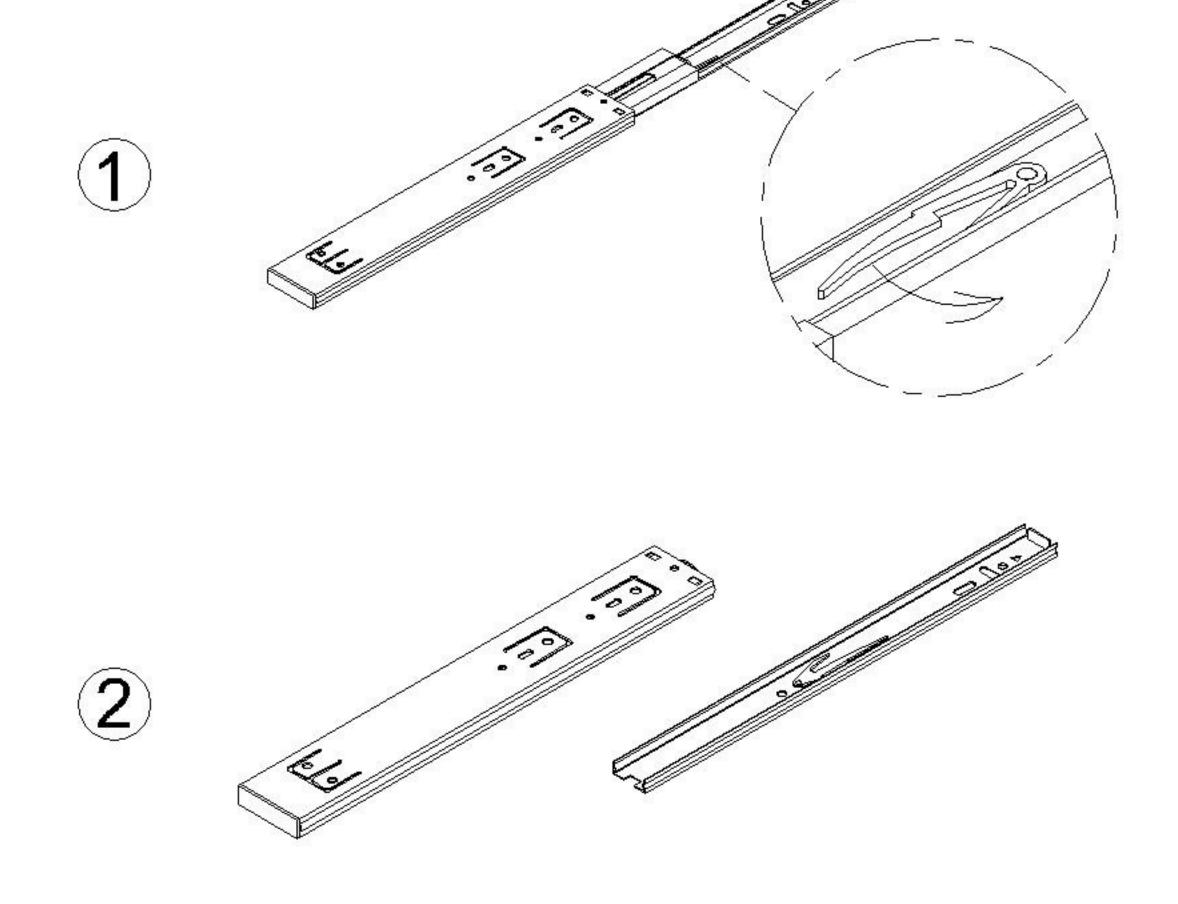
Disassemble the Runner (U) to 2 parts. Fix 1 part on the Left & Right Side Panel (B & C) and fix the other part on the Left & Right Drawer Side (I & L).
