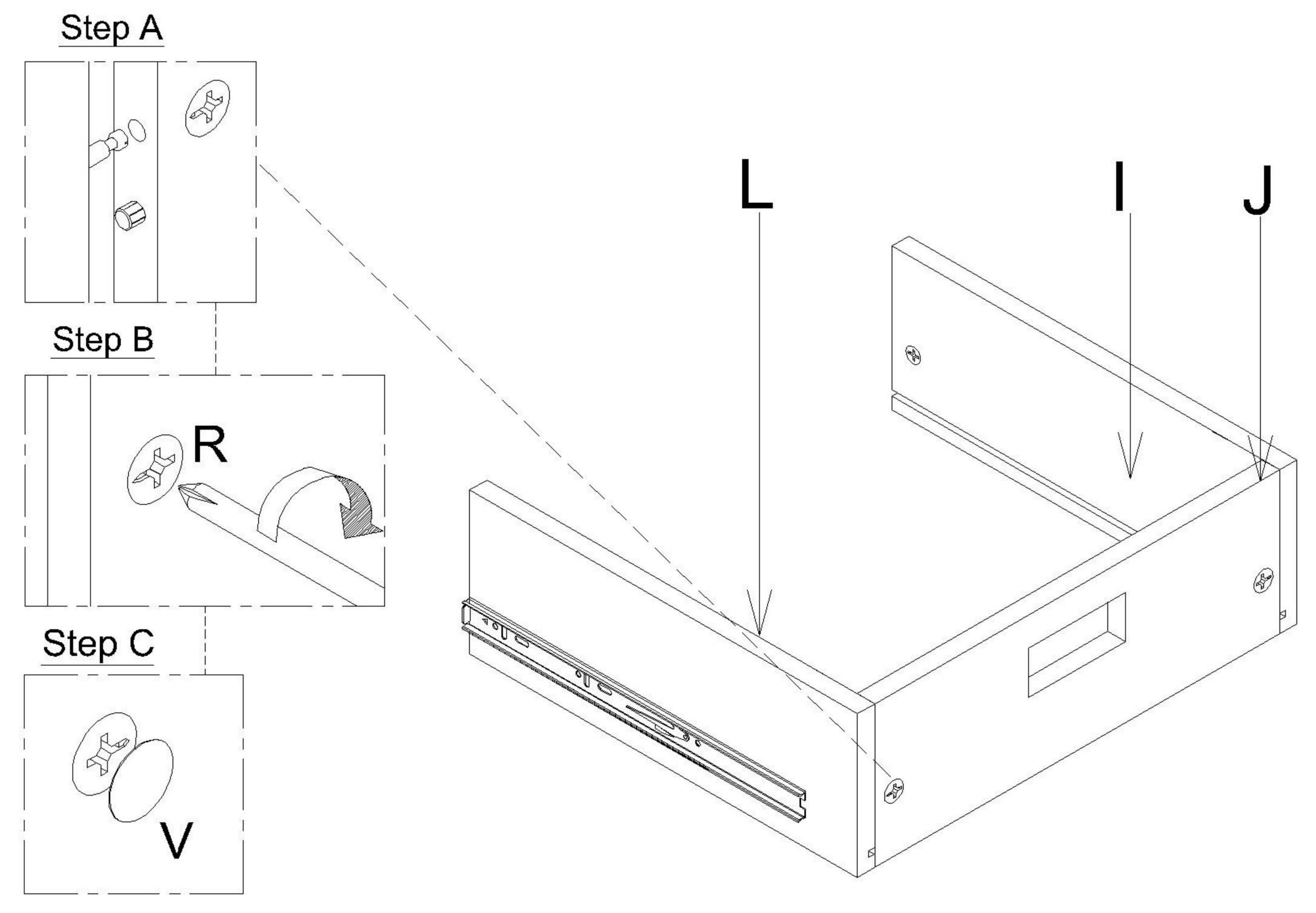
Slot Drawer Base (K) into corresponding grooves. Attach Drawer Front (H) to Drawer Box and secure with the Cam Lock (R) attached in the Step 12. Cover Cam Lock (R) with Cam Lock Cover (V).
