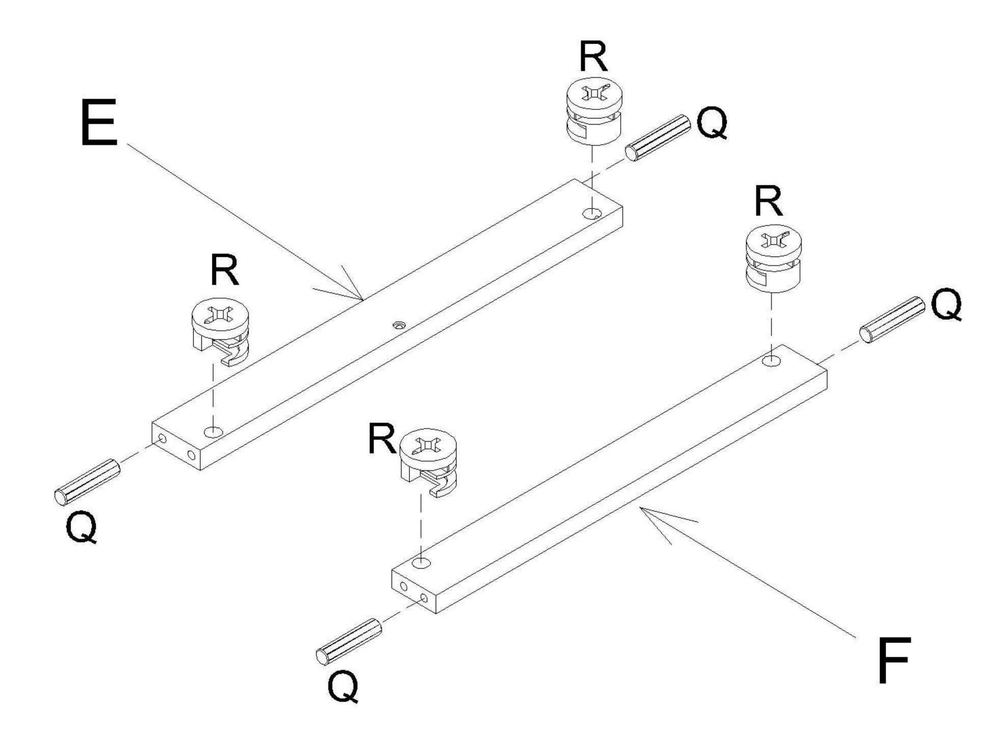
Attach Top Bar (E) & Center Bar (F) to Left Side Panel (B) and secure the Cam Lock (R) attached in the Step 5. Attach Bottom Panel (D) to Left Side Panel (B) and secure the Cam Lock (R) attached in Step 4. Cover Cam Lock (R) with Cam Lock Cover (V).
