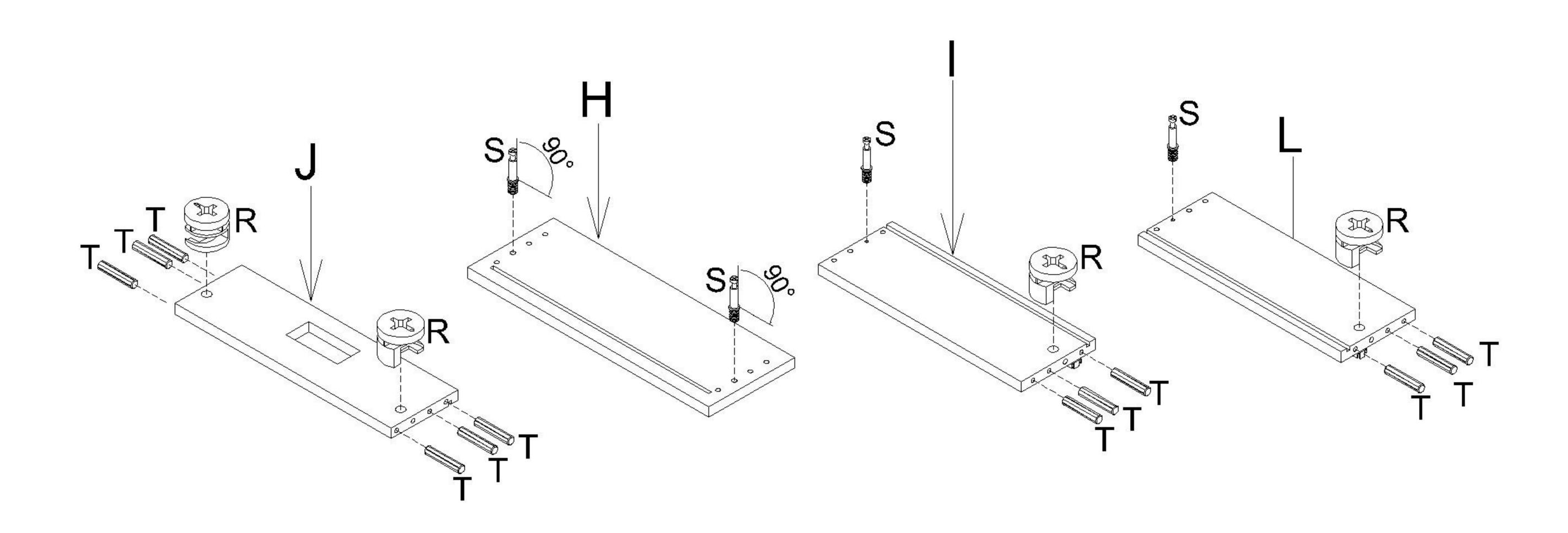
Attach Drawer Back (J) to Left & Right Drawer Side (I & L) and secure with the Cam Lock (R) attached in the Step 12. Cover Cam Lock (R) with Cam Lock Cover (V).
