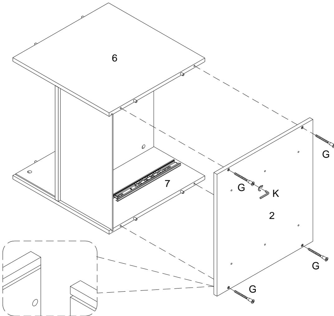
Using screw (G) attach part (2) to parts (6,7) with Hex key (K) as per diagram.
