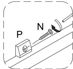
Using screw (N) secure plastic wedge (P) with Philips head screwdriver as per diagram.
