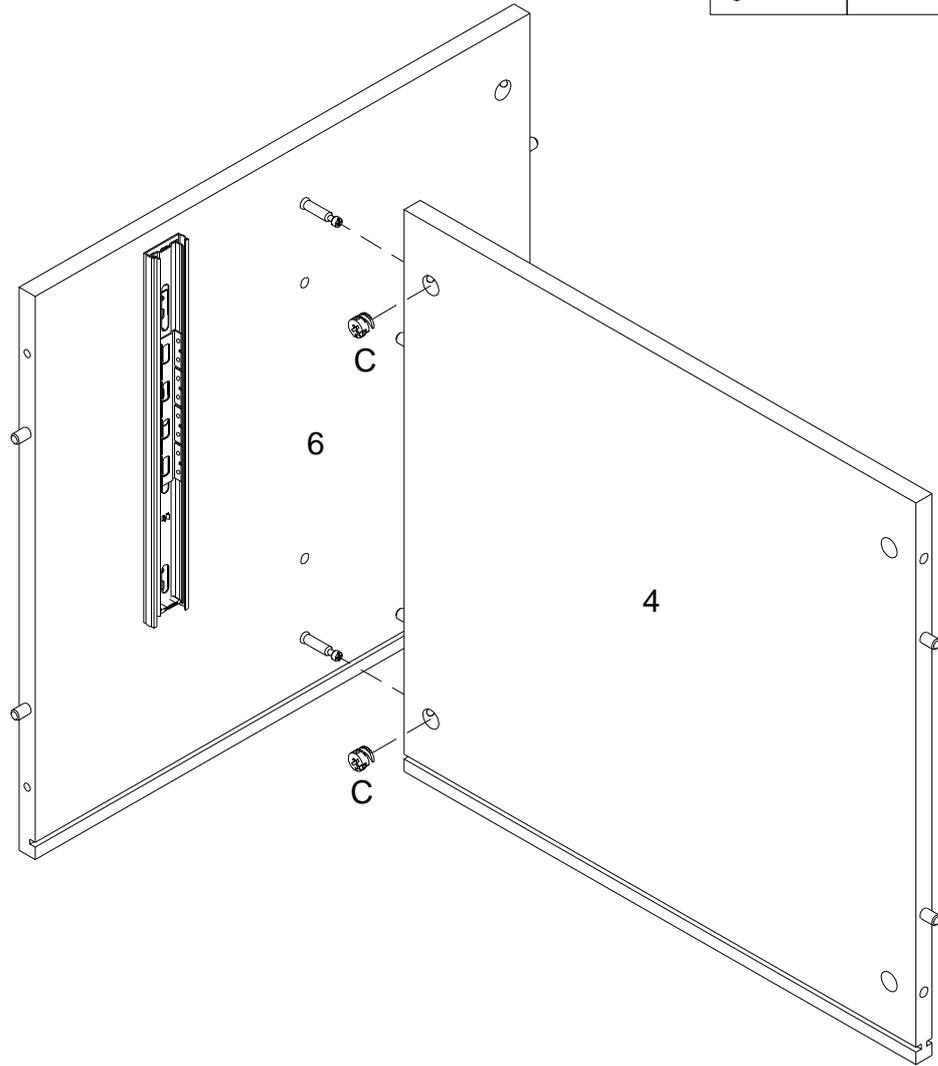
Using Cam lock(C) secure part (4) to part (6) with Philips head screwdriver as per diagram.
