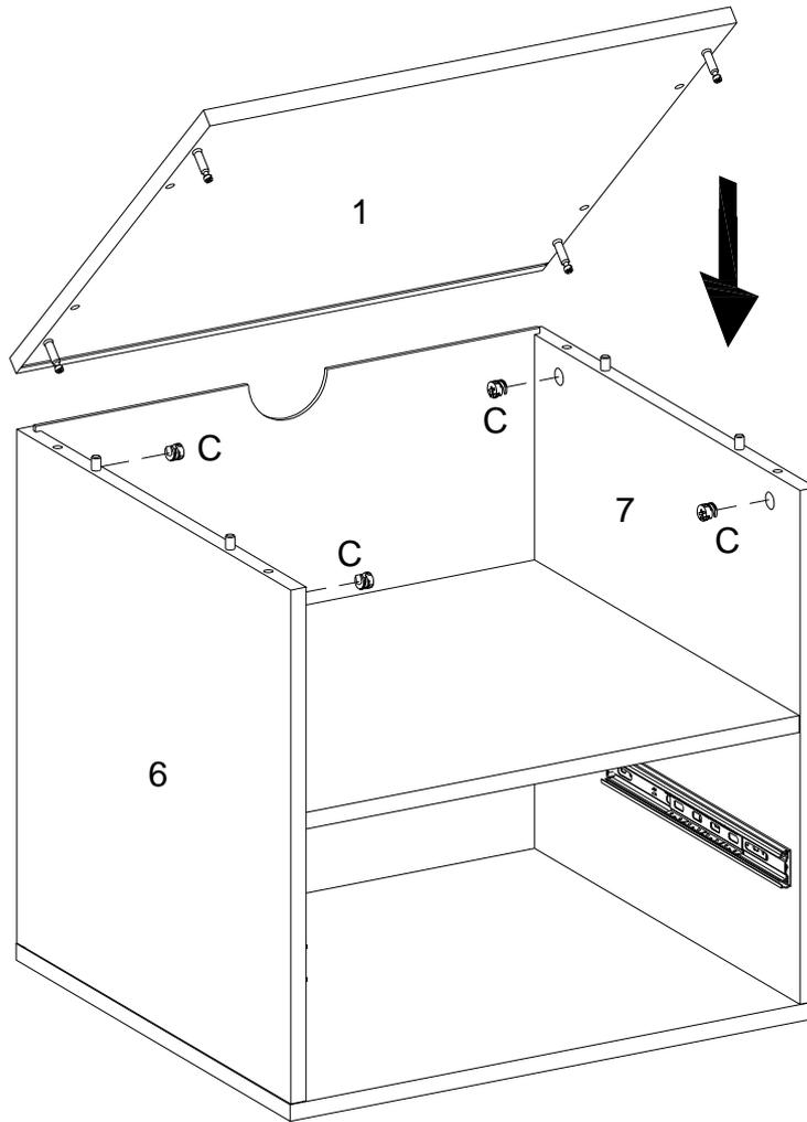
Using cam lock (C) secure part (1) into parts (6,7) with Philips head screwdriver as per diagram.
