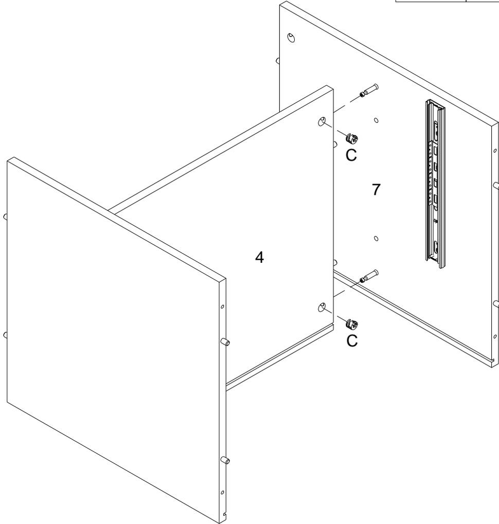
Using Cam lock(C) secure part (4) to part (7) with Philips head screwdriver as per diagram.
