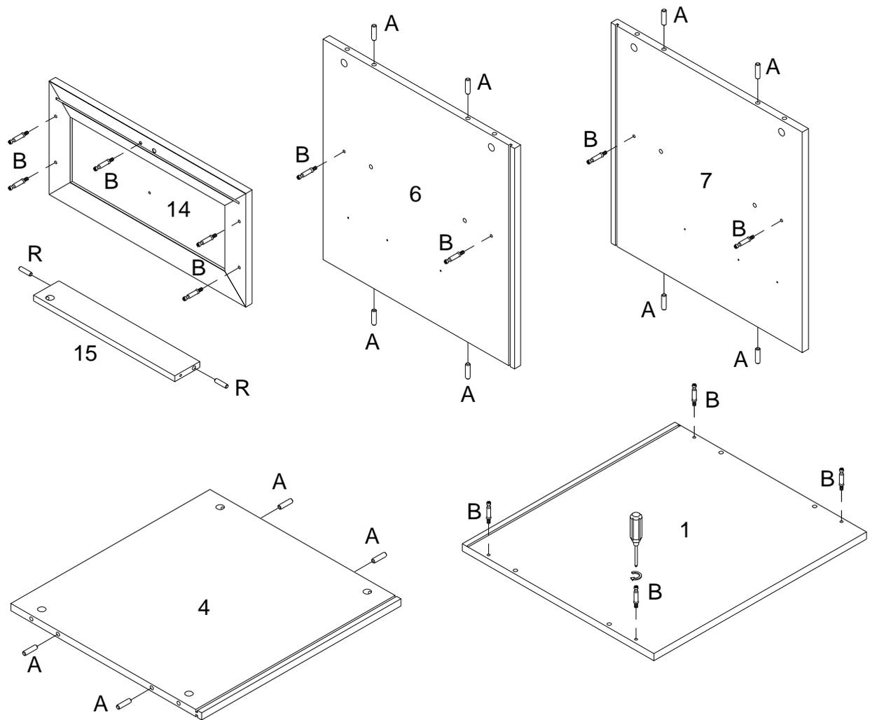
Insert wooden dowel (A) into parts (4,6,7) and wooden dowel (R) into part (15) ,then secure cam bolt (B) into parts (1,6,7,14) with Philips head screwdriver as per diagram.
