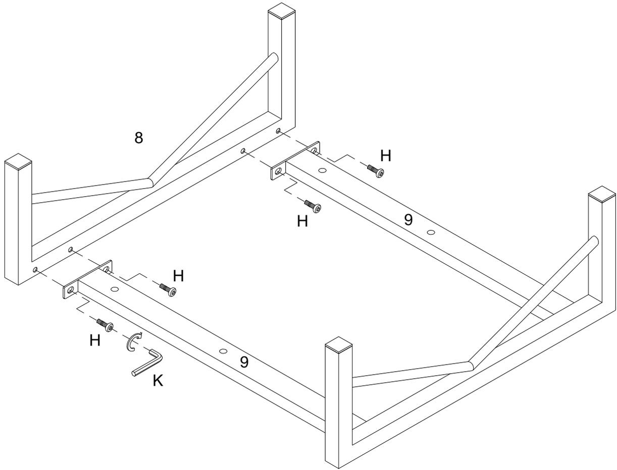
Using bolt (H) attach part (9) into part (8) with Hex key (K) as per diagram.
