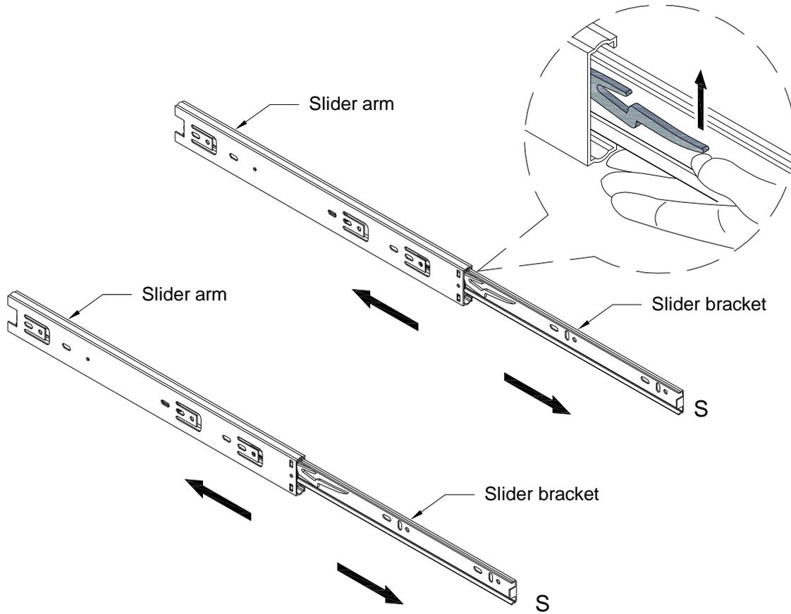
Pick up the slider arm (S) and separate the slide runner for the following Steps. Extend the slide runner all the way forward, press the plastic release lever of the slider arm up and pull the slide runner complete out .
