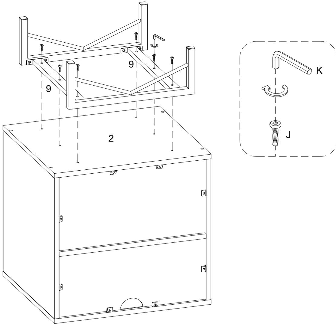
Using bolt (J) attach part (9) into part (2) with Hex key (K) as per diagram.
