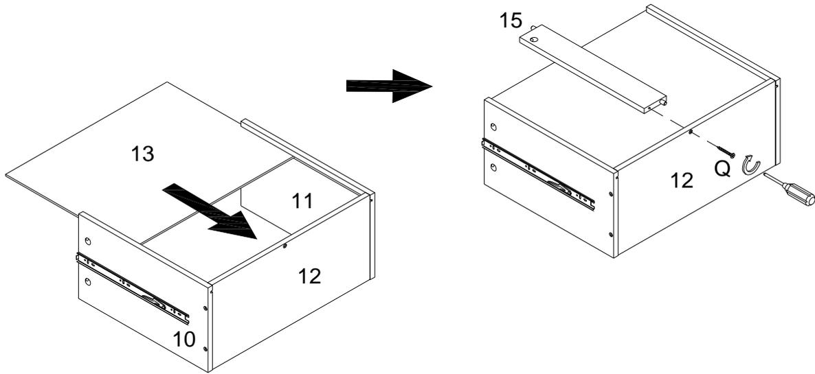
Put part (13) as per diagram. then use screw (Q) attach part (15) to part (12) with Philips head screwdriver as per diagram.
