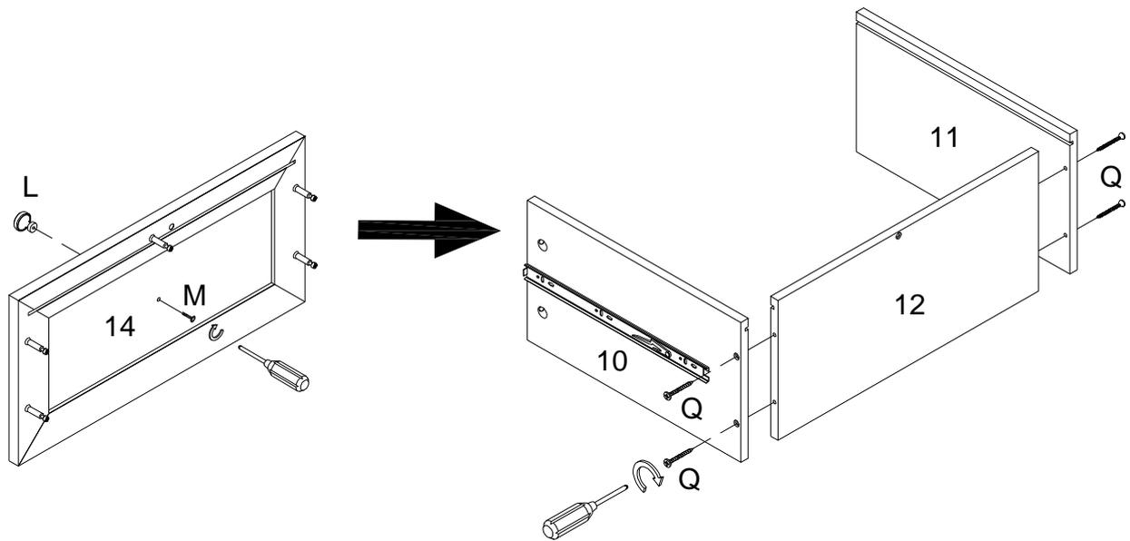
Using handle bolt (M) secure handle (L) to part (14) ,then using screw(Q) attach parts (10,11) to part (12) with Philips head screwdriver as per diagram.
