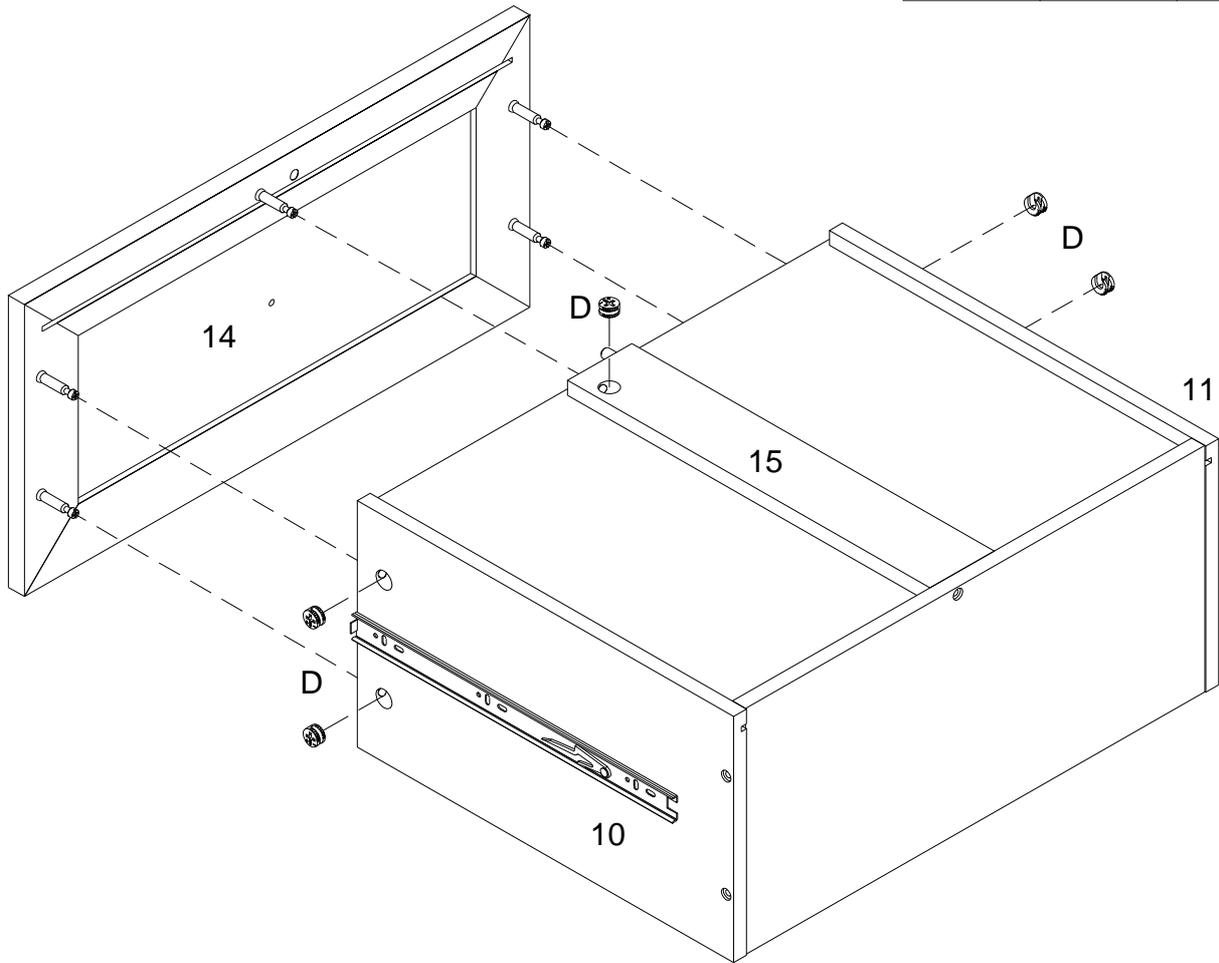
Using Cam lock(D) secure part (14) to parts (10,11,15) with Philips head screwdriver as per diagram.
