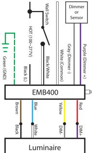
NOTE: Dimming leads from EMB400 to LED Driver must be attached to the DIM+ and DIM- wires of the luminaire regardless of the use of any other sensors or control systems.
