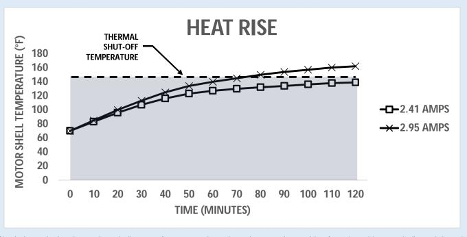
The Shaded area in the charts above indicate performance points where the pump is capable of running without periodic cool down based on current draw. Performance points in the unshaded areas require periodic shut down for motor cooling. Some applications require maximum flows at high pressures for relatively short periods, so an explanation of thermal protection follows:
