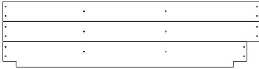
CT01 COUNTER TOP - W2A05008 (x1) 13/16"x11 1/8"x43 1/16" (21x283x1093)
