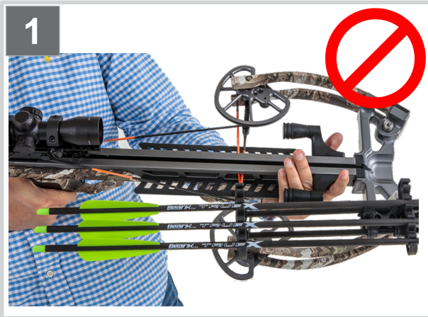
Pictures 1-4. Improper Hand Position – with your fore-grip positioned as shown you will have a severed hand or finger amputation
