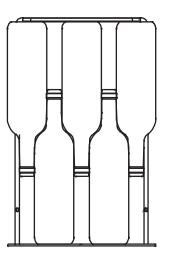
Store wine in sealed bottles only Avoid overloading Storing little or no product can cause excessive condensation
