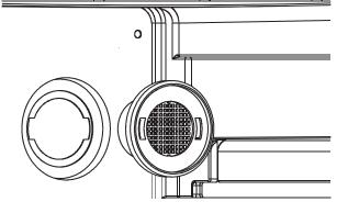
Rotate filter 1/4 turn to lock in place
