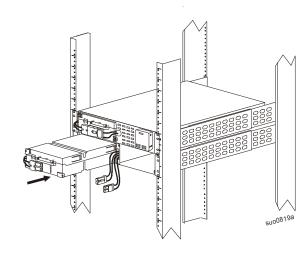
Slide the left hand side battery module into the XLBP.
