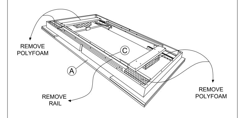
STEP 2: Remove all polyfoam and then remove all the bolt covers on table legs (B).
