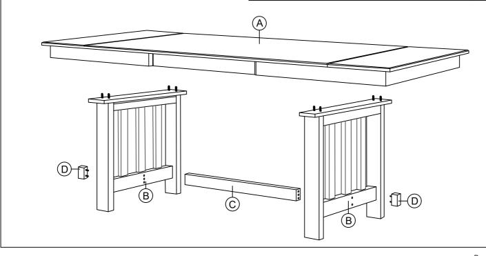
STEP 1 : Place the table top (A) upside down on a flat and clean surface. Remove all polyfoam & rail (C).
