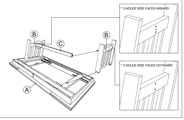
STEP 5 : Assemble the Table Legs (B) to the Table Top (A) by using the Wrench (7) and the hardware Nut (3), Spring Washer (4) & Flat Washer (5).
