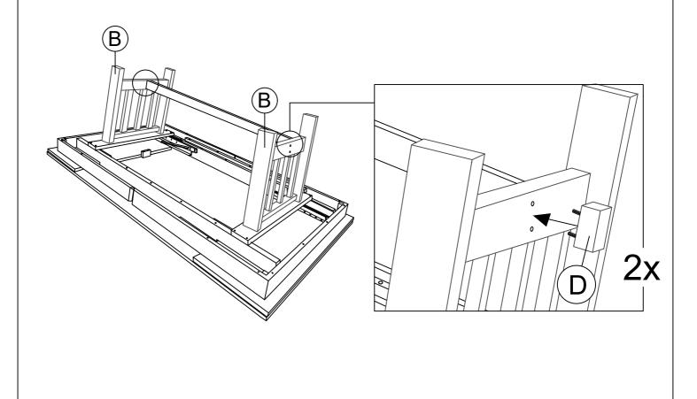
STEP 8 : Remove and discard the wood blocks with screwdriver to operate the table leaves.
