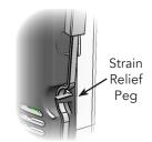
**Power up the panel** by inserting the power supply barrel into the power jack on the side. Route the power cable under the strain relief peg.
