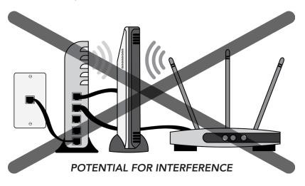
• Put some space between the panel and the home router. A 6-foot cable is included for this purpose.
