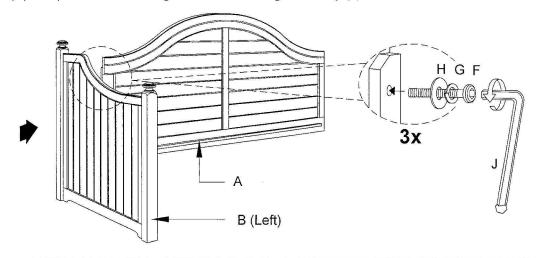
Attached Side Frame (C) (Right) to Back Panel (A) by inserting JCBC Bolt (F) with Spring Washer (G) and Flat Washer (H) into provided holes. Do not tighten the bolts. Insert Front Rail (D) to Side Frame (B) (Left). Repeat the same process to Side Frame (C) (Right). Then tighten all the bolts using Allen Key (J).
