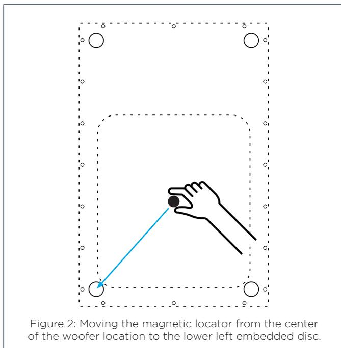
**about 12mm.** This typically results in a more accurate pinpointing of where the embedded discs are and will result in more accurate measurements.
