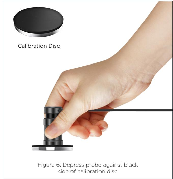
Figure 6: Depress probe against black side of calibration disc
