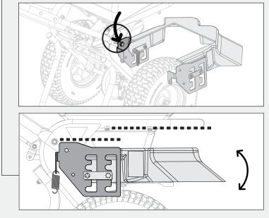
3c. Using the mounting bracket as a template, mark the center point for drilling (marked with a "Z" here) with a set punch or marker.
