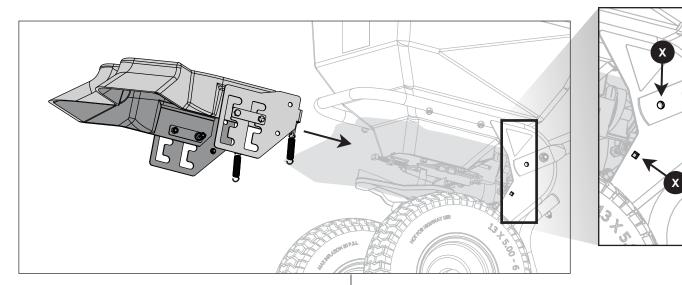
5. On both sides of the spreader, **LOOSELY** attach the deflector with the hex bolt (A), two washers (B) and lock nut (C) that were removed on Step 2.
