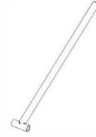
R04 TIGE DE PIVOT - A4M02784 (x1) 1/2"x1 7/16"x12 1/4" (12x36x312)
