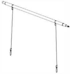
S01 ASSEMBLAGE DE BROCHE - A4M02150 (x1) 1 3/16"x37 5/8" (x30x955)
