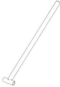
R04 TIGE DE PIVOT -A4M02784 (x1) 1/2"x1 7/16"x12 1/4" (12.0x36x312)
