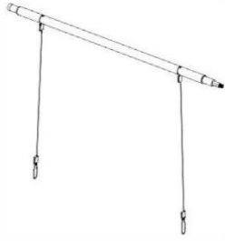
S01 ASSEMBLAGE DE BROCHE -A4M02150 (x1) 1 3/16"x37 5/8" (30x955)
