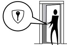
Right Hand " RH ", Hinges Right, Open Inward.
