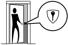
Left Hand " LH ", Hinges Left, Open Inward.
