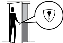
Left Hand Reverse " LHR ", Hinges Left, Open Outward.
