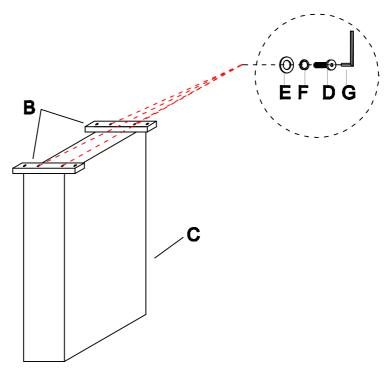
Attach Connecting Plate(B) to Top(A) by using Bolt(D), Flat Washer(E), Spring Washer(F) and Allen Wrench(G) as shown.
