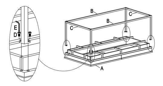
With assistance from your adult partners, turn the Table right way up. Adjust the Pre-installed Levelers on the bottom of Leg (B) until the Table is level with the ground.
