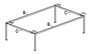
Fix Leg (B) and Rail (C) using Bolt (D) with Allen Key (F).
