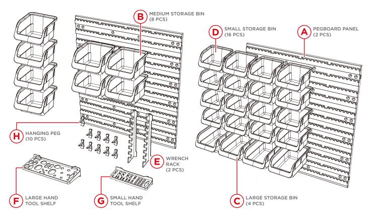
This item does not include any mounting hardware. Please use appropriately sized screws (at least 3-inches long) depending on the wall material. Use longer screws for softer wall materials.
