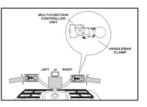
To release the MC900B controller from the mounting bezel, insert a small jewellers screwdriver into the left / right slots of the bezel.
