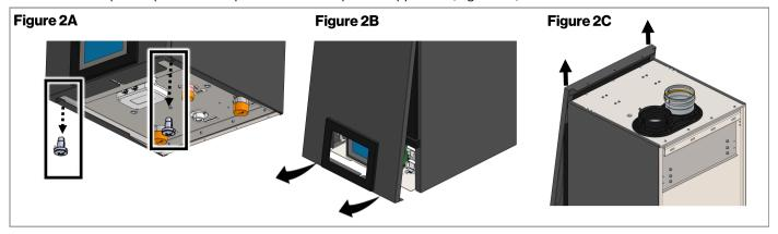
5. **RCB301AN/RCB399AN:** Use a Phillips head screw driver to remove three (3) screws holding left side panel (Figure 3A). Rotate the side panel out (Figure 3B), push the panel up to clear the cutout located on back side of boiler, and pull the side panel out (Figure 3C).
