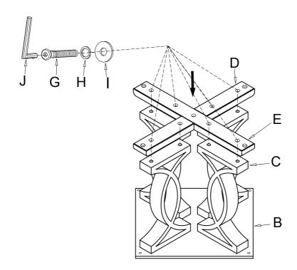
Place the Table Top (A) upside down on the smooth carpet surface. Tighten the Joint Panel (B) to the Table Top (A) by Bolt (F), Lock Washer (H) and Flat Washer (I) with Allen Wrench (J).
