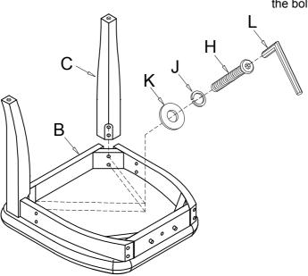
Place the Chair Back (A) with Seat (B) on the smooth carpet surface. Attach the Chair Back (A) with Seat (B) by Bolt (I), Lock Washer (J) and Flat Washer (K) with Allen Wrench (L). Then tighten Chair Back (A) and Seat (B) by Bolt (E), Lock Washer (F) and Flat Washer (G) with Allen Wrench (L).
