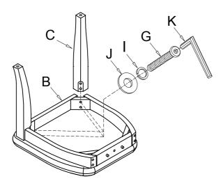
Take the Allen Wrench, and turn the bolts until the legs are secured. DO NOT TIGHTEN COMPLETELY. Stop when you feel you are adding force to tighten the bolt.
