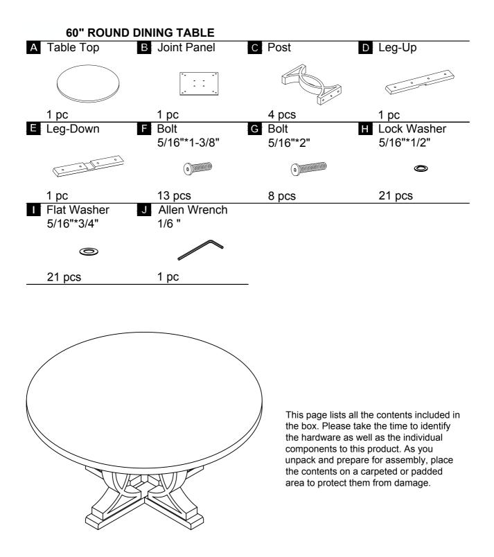
Place the Leg-Up (D) and Leg-Down (E) upside down on the smooth carpet surface. Tighten the Leg (D&E) by Bolt (F), Lock Washer (H) and Flat Washer (I) with Allen Wrench (J).
